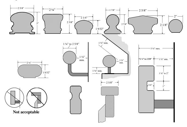
Other shapes may be acceptable if they provide an equivalent gripping surface. Do not use these shapes to make your hand rails and expect that the hand rail will automatically pass inspection, check with Building Inspector to see if the shape you want to make will work.
