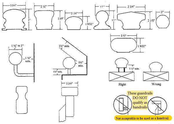
Other shapes may be acceptable if they provide an equivalent gripping surface. Do not use these shapes to make your handrails and expect that the handrail will automatically pass inspection, check with Building Inspector to see if the shape you want to make will work.
