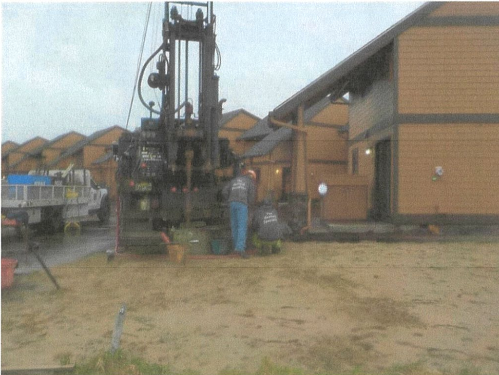
Photo 2 – View of the drill rig set up at the location of Boring B-1.
