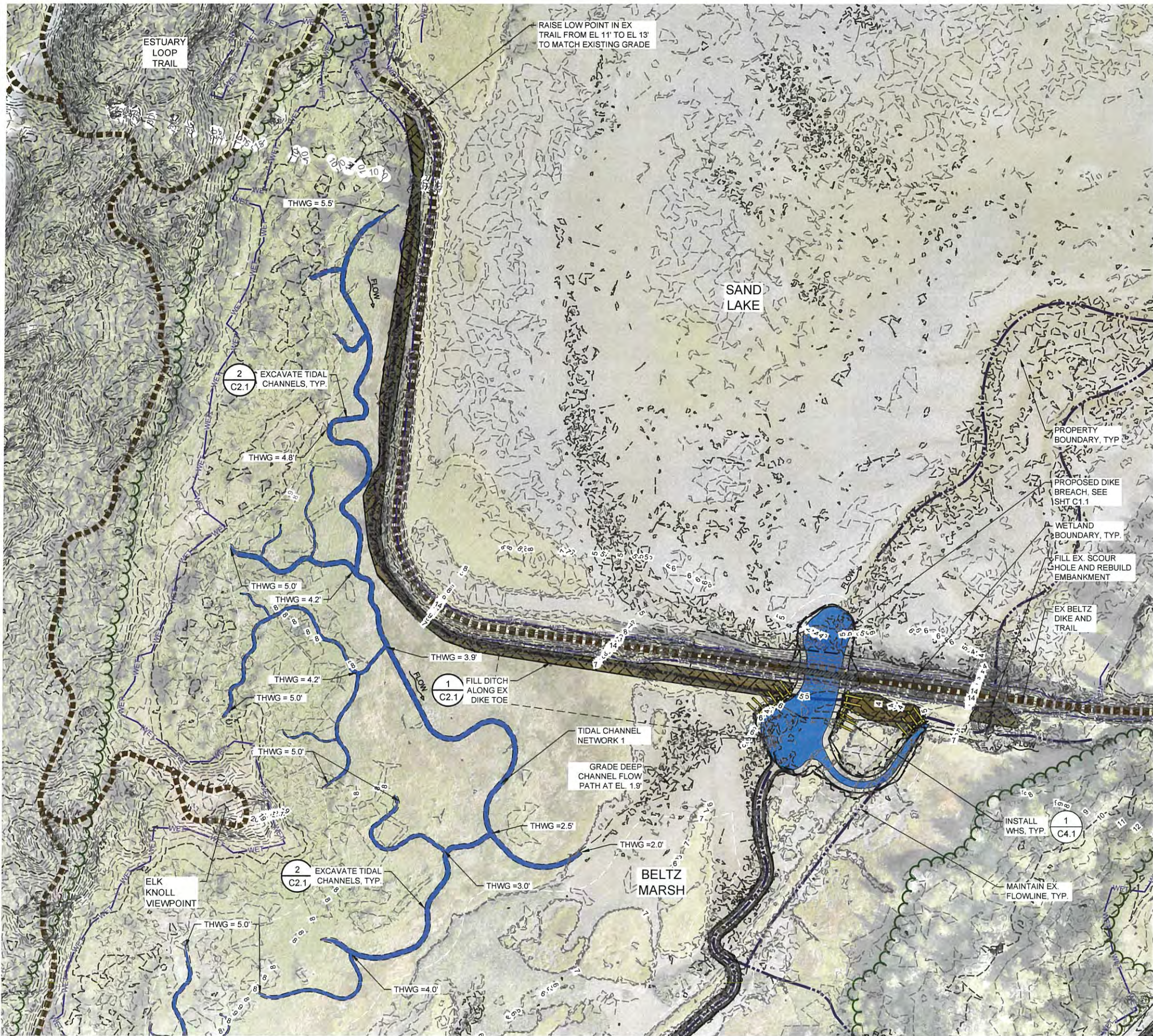
CHANNEL AND DITCH GRADING ENLARGEMENT - 1 PLAN
