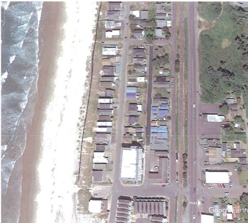
Figure 3. Naturally buried revetment near Rockaway Beach (revetment edge represented by black line)
