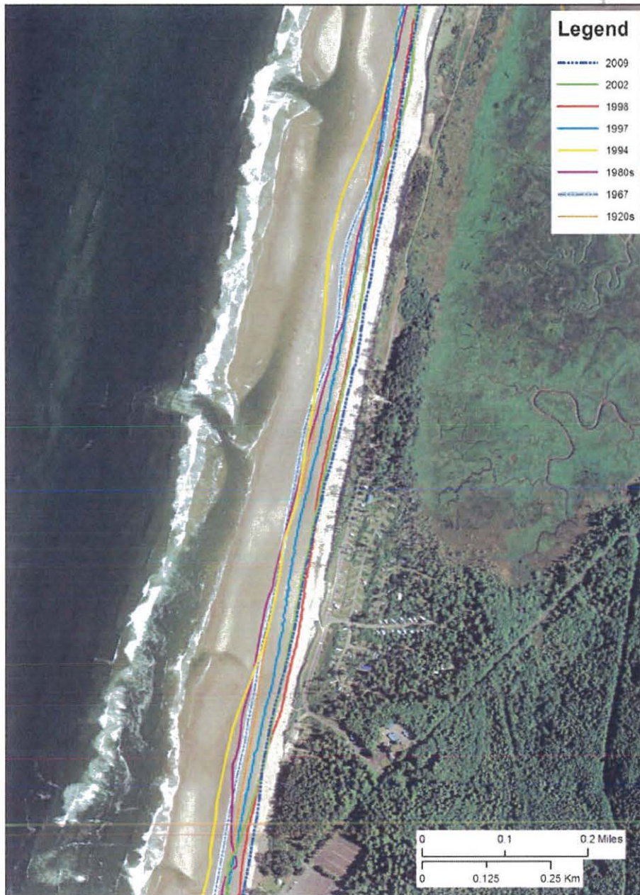
Figure 2-20. Historical and contemporary shoreline positions identified along the southern end of Netarts Spit, adjacent to Cape Lookout State Park. Note: The 1920s (1927/28) shoreline is derived from NOS T-sheets, 1967 and 1994 are from orthorectified aerial photographs, 1980s (1985/86) is from U.S. Geological Survey topographic maps, and 1997–2009 are derived from lidar.
