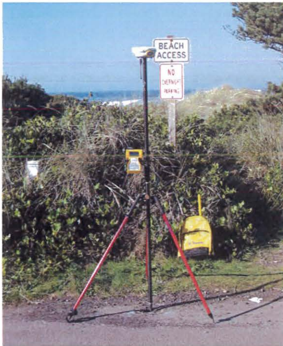
Figure 5. Static GPS occupations were used as part of a site calibration on selected benchmarks to derive a local coordinate system in the Rockaway littoral cell. GPS site calibration procedures involved occupying a benchmark for 180 epochs (typically at least 3 minutes or longer) and then processing the data in Trimble Geomatics Office software.
