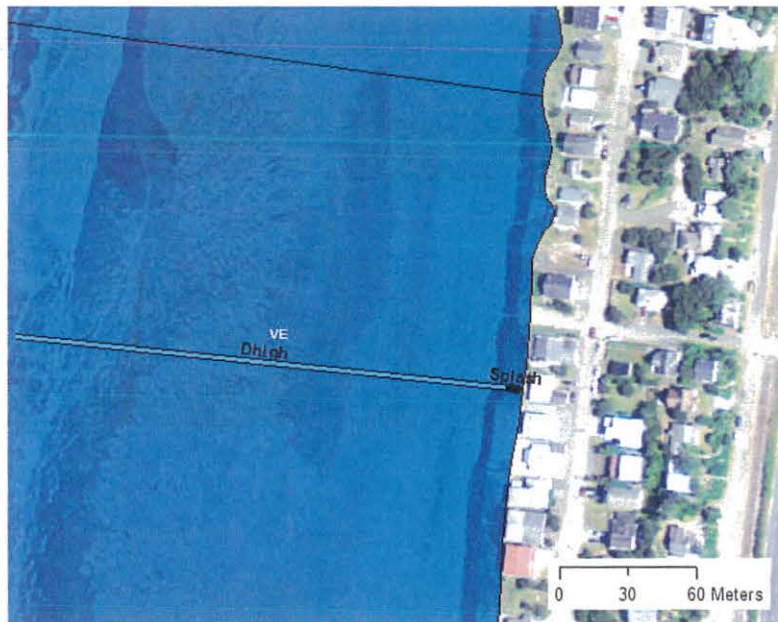
Figure 8-4. TILL 144 transect at Rockaway with overtopping splash zone. The short splash zone distance (black) was added to the extent of the VE zone.
