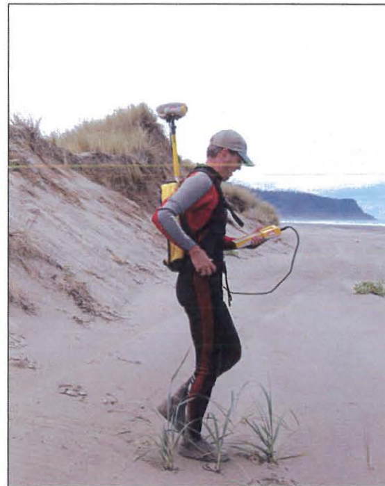
Figure 6. Profile survey undertaken near Neskowin using a Trimble 5800 GPS rover mounted on a backpack.
