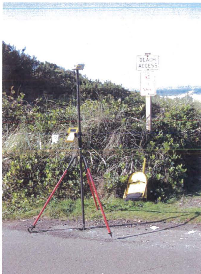
Figure 3-5. A 180-epoch calibration check is performed on a survey monument (Rock7) established in the Rockaway littoral cell in Tillamook County. This procedure is important for bringing the survey into a local coordinate system and for reducing errors associated with the GPS survey (photo: J. Allan, DOGAMI, 2004).
