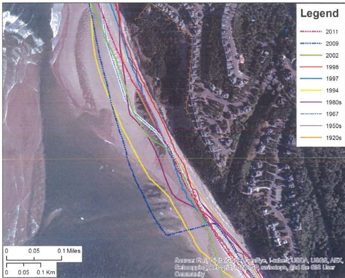
Figure 2-26. Historical shoreline positions identified along the toe of The Capes development near the mouth of Netarts Bay. Here we include one additional shoreline (2011) surveyed using GPS. Brown hashed line depicts the landslide headscarp.
