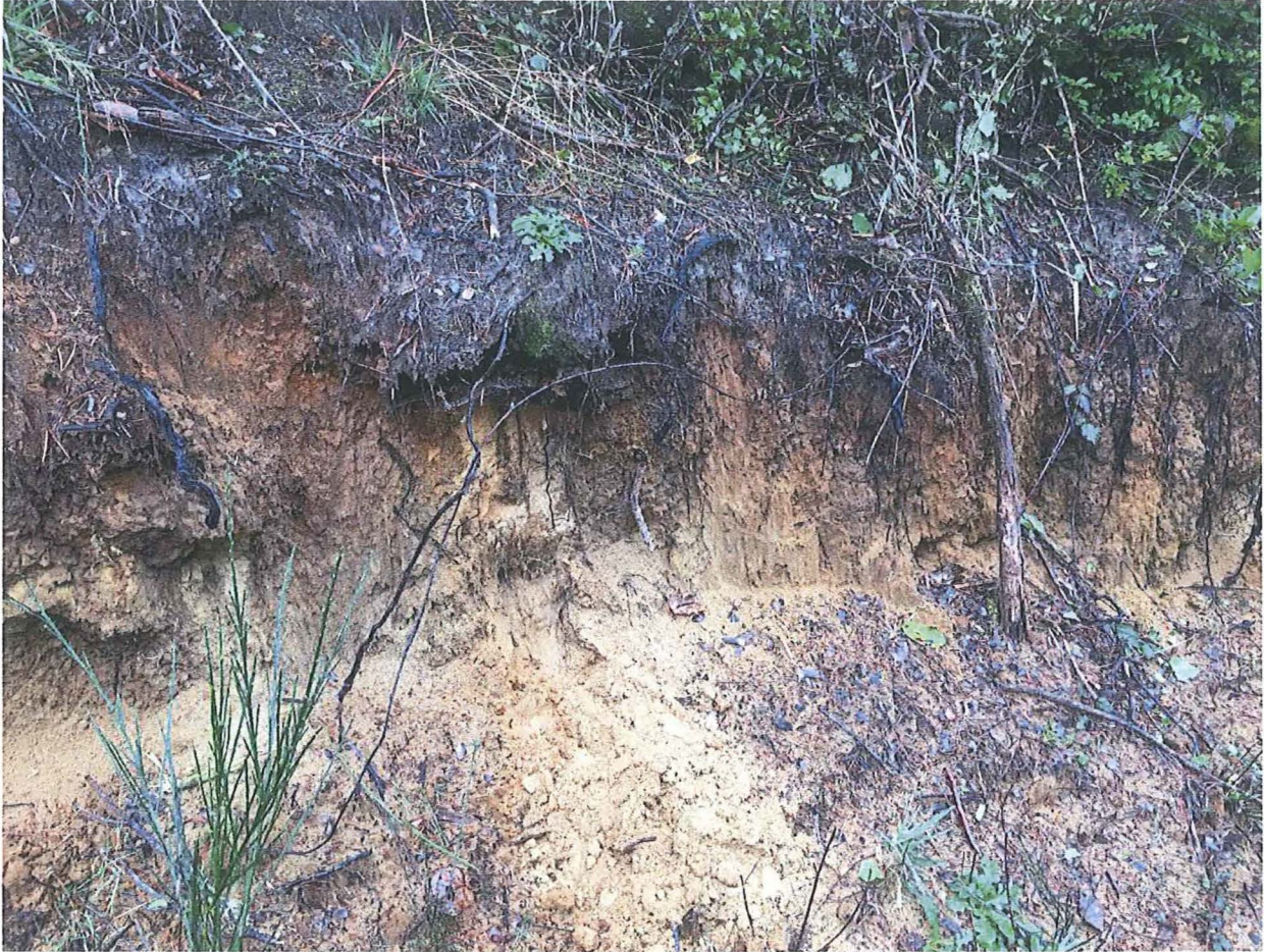
Image 2: 1-2 feet of soil was exposed at a roadcut approximately in the middle north of the site. Soil on the site is deep, fine sand with slight to moderate cementation.
