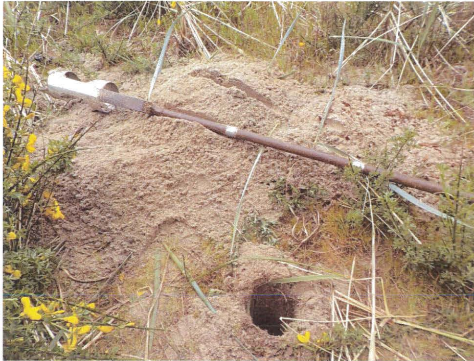
Photo 7 – View of the dune sand encountered in boring B-2 to a depth of approximately 13 feet below the ground surface.
