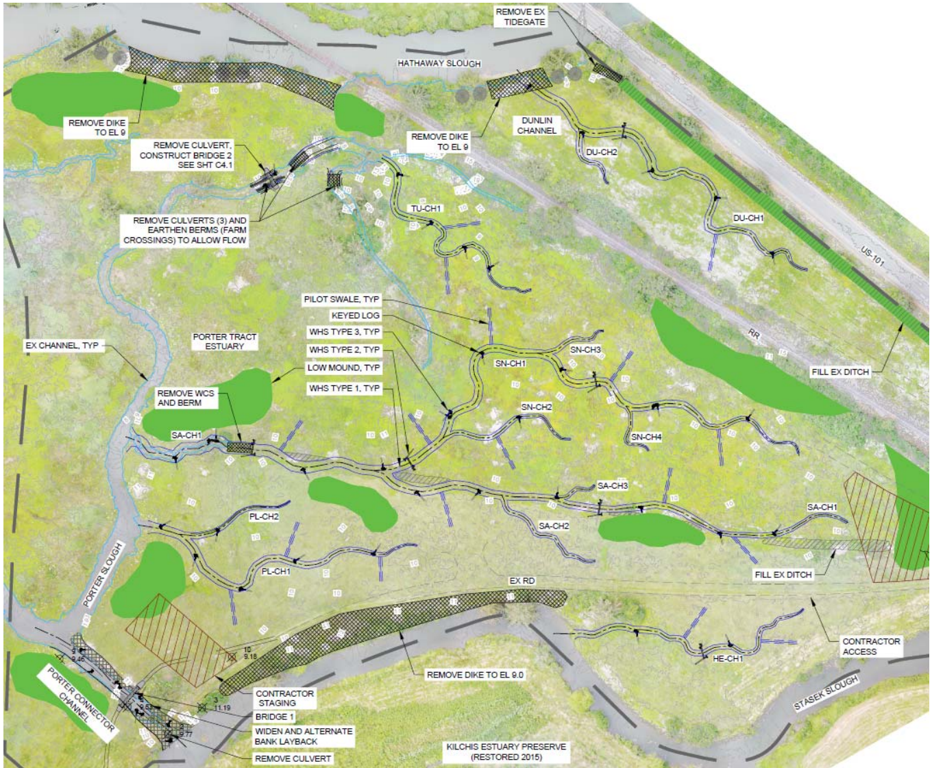
Figure 1 Porter Tract restoration site overview indicating restored channels, filled ditches, dike removals, new bridges, and low mounds.
