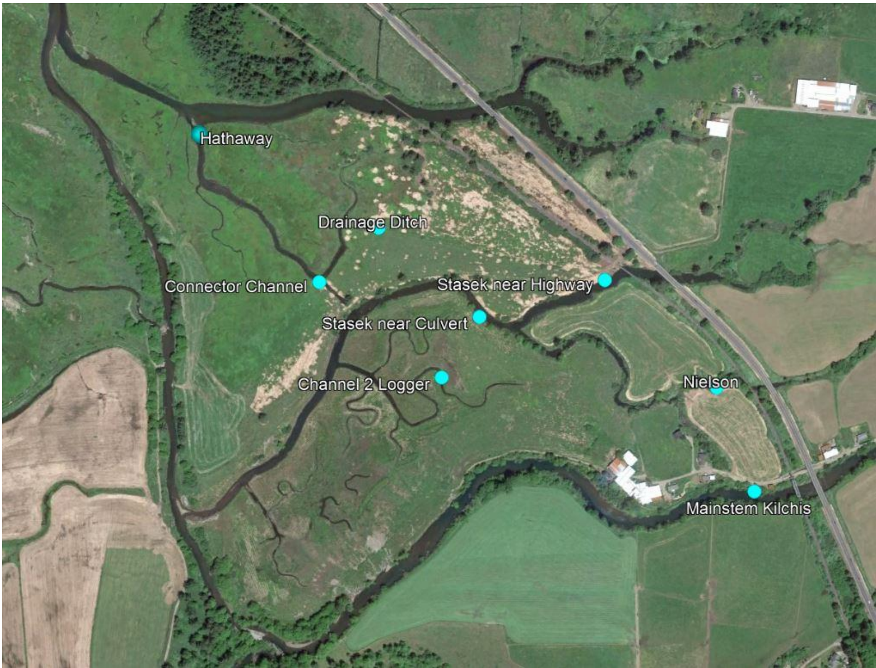
Figure 17. Locations of Water Level Loggers at Kilchis Preserve for Hydrologic Monitoring
