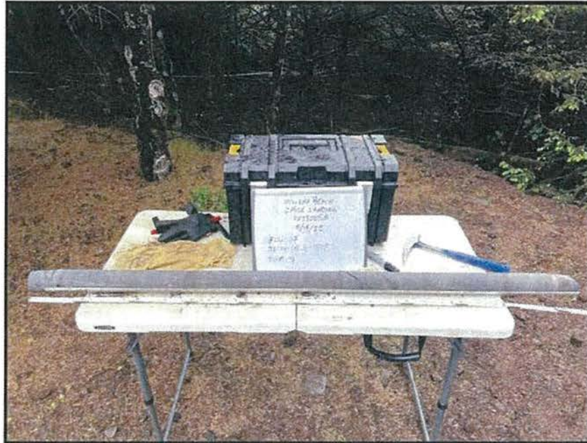
PHOTO 29: BORING B-1, CORE RUNE 17: 146.5 FT -151.5 FT
