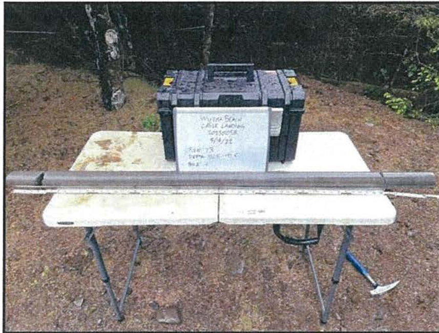
PHOTO 25: BORING B-1, CORE RUNE 13: 126.5 FT - 131.5 FT
