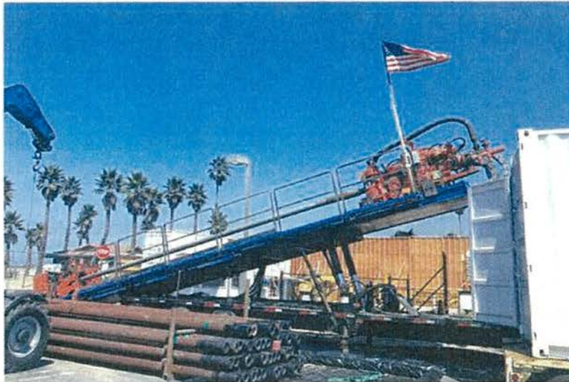
Figure 1: Example of HDD Rig
