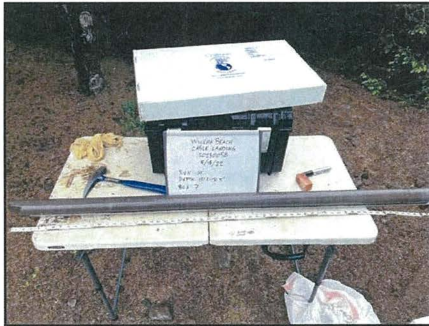
PHOTO 26: BORING B-1, CORE RUN 14: 131.5 FT - 136.5 FT
