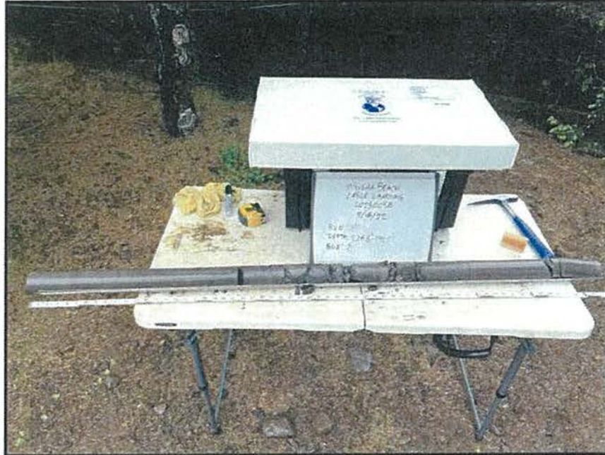
PHOTO 27: BORING B-1, CORE RUN 15: 136.5 FT -141.5 FT
