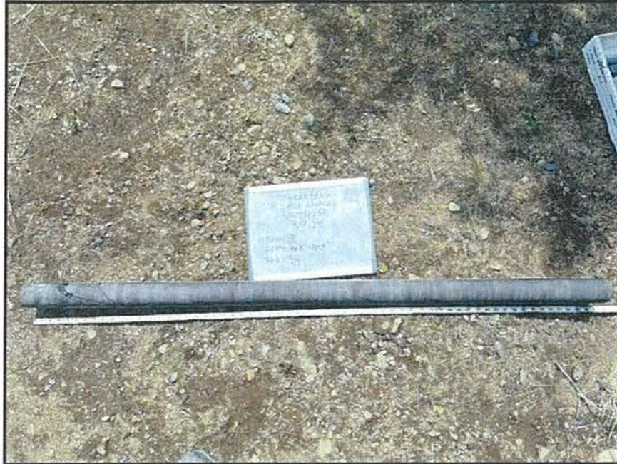
PHOTO 19: BORING B-1, CORE RUN 7: 96.5 FT -101.5 FT
