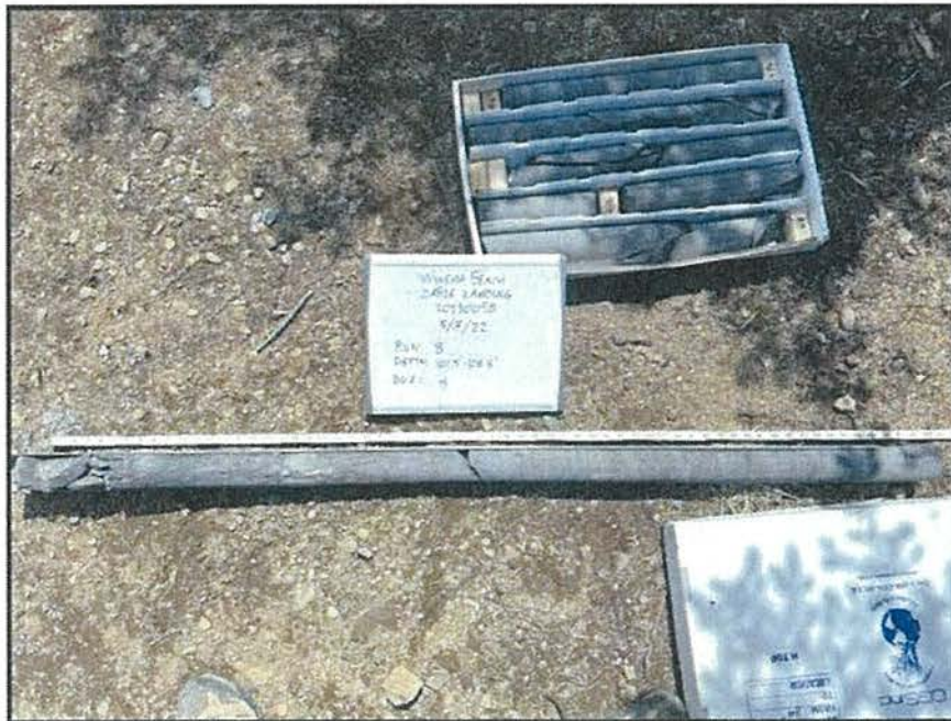
PHOTO 20: BORING B-1, CORE RUN 8: 101.5 FT - 106.5 FT
