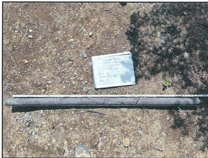
PHOTO 18: BORING B-1, CORE RUN 6: 91.5 FT - 96.5 FT
