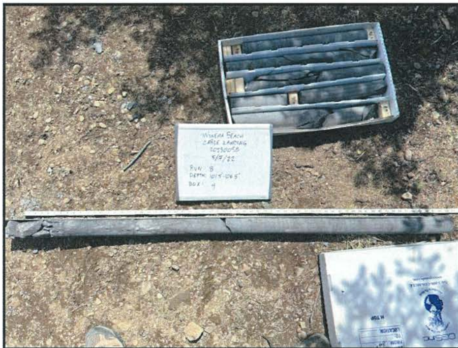
PHOTO 20: BORING B-1, CORE RUN 8: 101.5 FT - 106.5 FT
