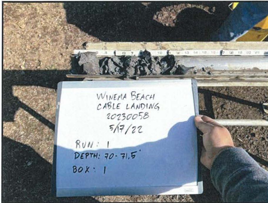
PHOTO 13: BORING B-1, CORE RUNE 1: 70 FT -71.5 FT
