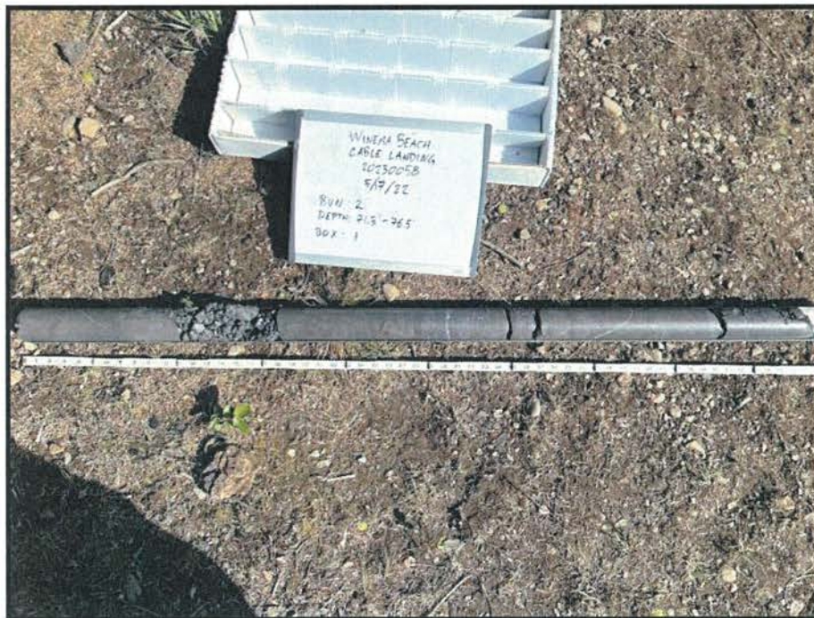
PHOTO 14: BORING B-1, CORE RUN 2: 71.5 FT - 76.5 FT
