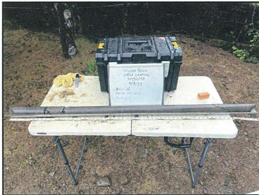
PHOTO 28: BORING B-1, CORE RUN 16: 141.5 FT - 146.5 FT
