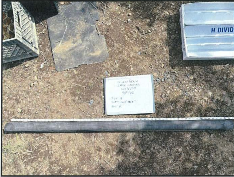
PHOTO 23: BORING B-1, CORE RUN 11: 116.5 FT -121.5 FT
