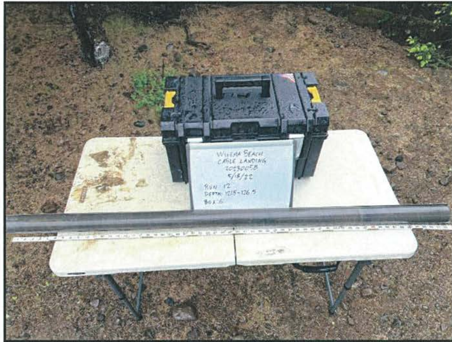
PHOTO 24: BORING B-1, CORE RUN 12: 121.5 FT - 126.5 FT
