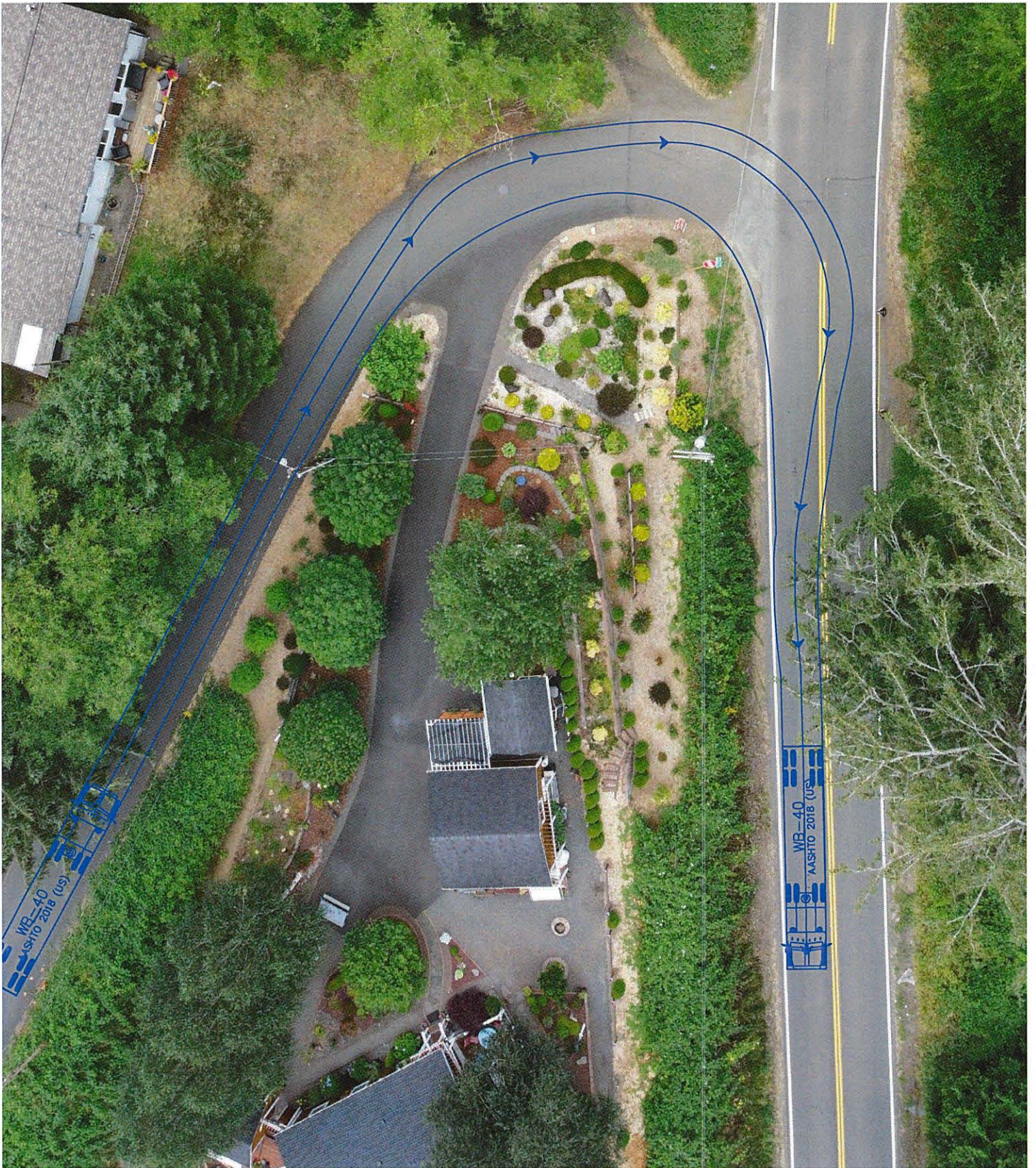
WB-40 Tractor Trailer Using Both Lanes (Downhill)
