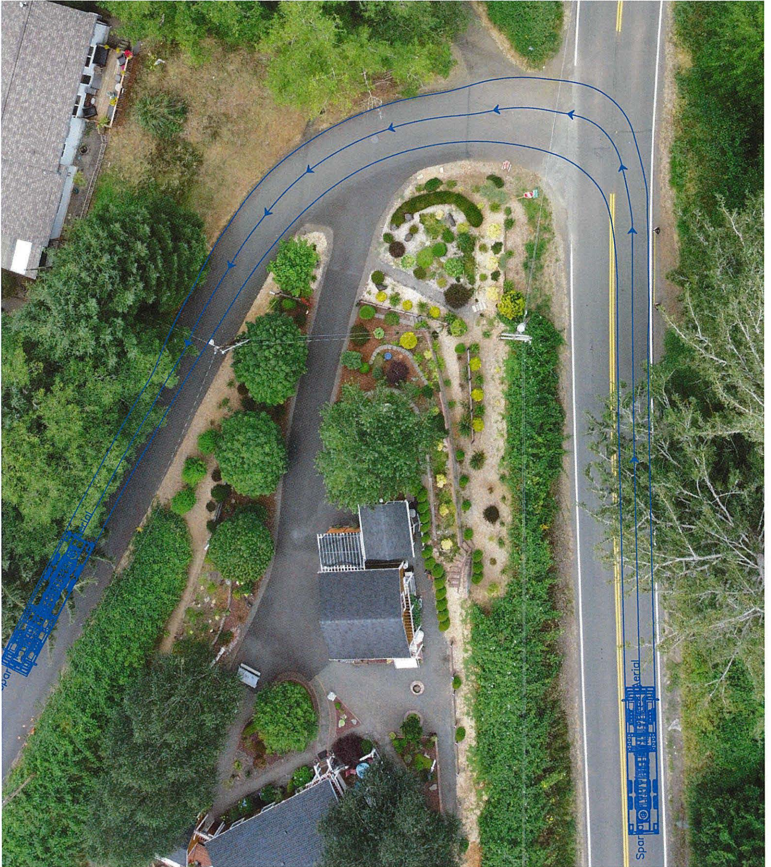
Fire Apparatus Using Both Lanes (Uphill)
