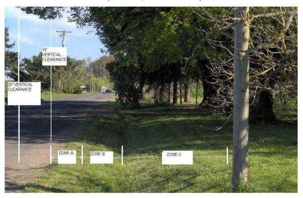
Zone A – Edge of Road (asphalt/gravel driving surface) to Shoulder.
