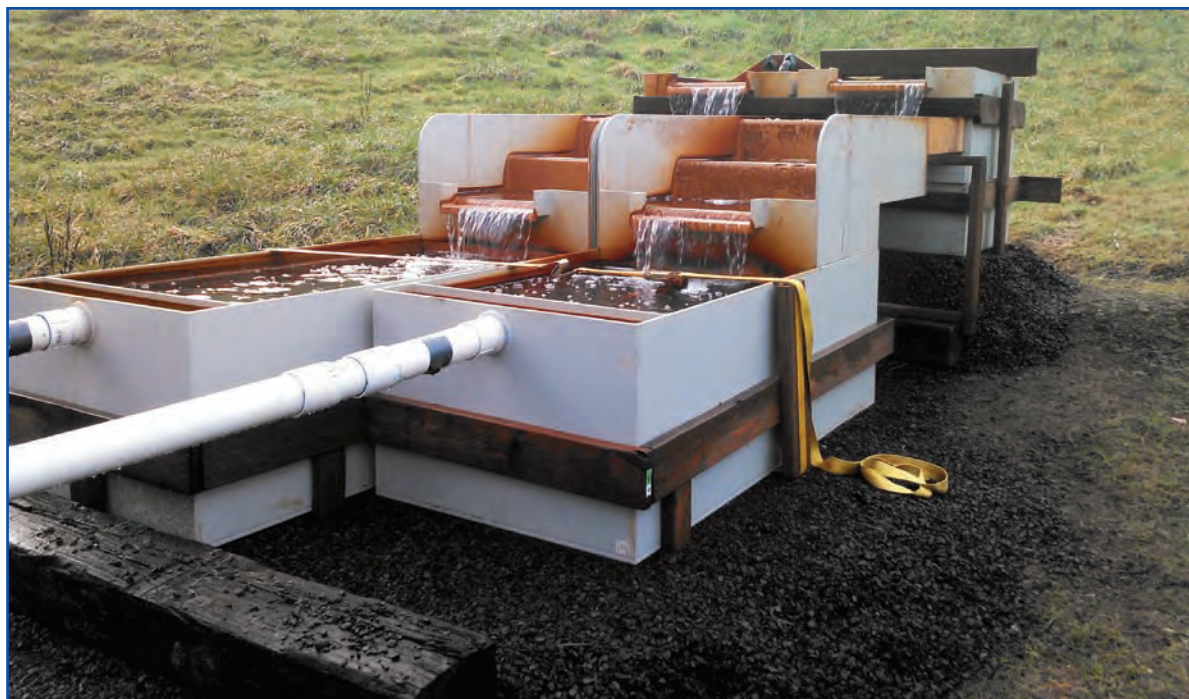
The cascade aeration trial aims to decrease iron in the leachate.
